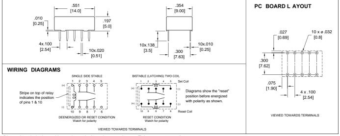
Dimensions in inches with metric equivalents in parentheses. Tolerance:  $\pm 0.010"$
